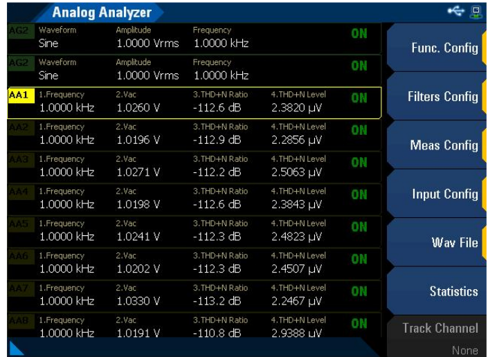
Figure 4. The U8903B's GUI, showing 8 analyzer channel measurements.
